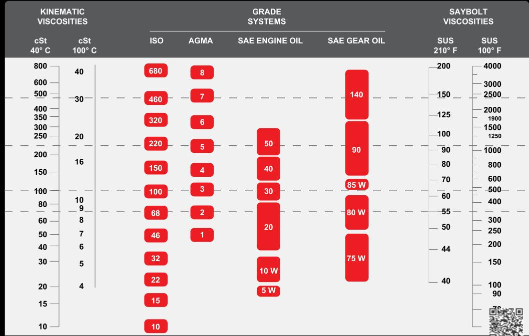
Viscosities can be related horizontally only, For example, the following oils have similar viscosities: ISO 460, AGMA 7 and SAE GEAR OIL 140. The viscosity/temperature relationships are based on 95 VI oils and are unable mono grade engine oils, gear oils and other 95 VI oils. Crankcase oils and gear oils are based on 100° C viscosity. The "W" grades are classified on low temperature properties. ISO oils and AGMA grades are based on 40° C viscosity.
