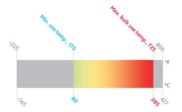
Eastman Therminol® 75 heat transfer fluid offers excellent thermal stability. It was developed for use at temperatures up to 385°C (725°F) in typical liquid phase heat transfer systems that operate at low pressure. Static pressure of about 1½ atmospheres should maintain the liquid phase at high temperatures.
