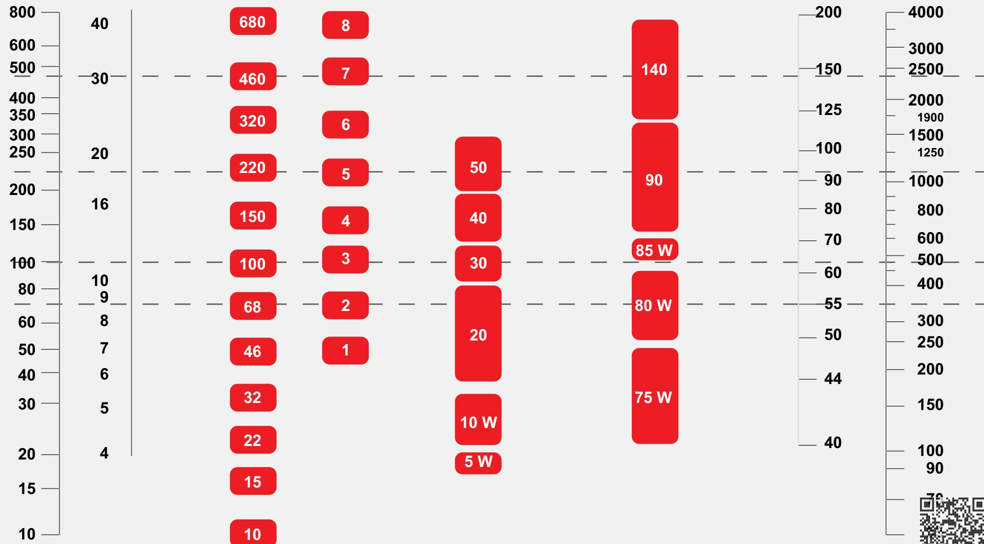
Viscosities can be related horizontally only. For example, the following oils have similar viscosities: ISO 460, AGMA 7 and SAE GEAR OIL 140. The viscosity/temperature relationships are based on 95 VI oils and are used for mono grade engine oils, gear oils and other 95 VI oils. Crankcase oils and gear oils are based on 100° C viscosity. The "W" grades are classified on low temperature properties. ISO oils and AGMA grades are based on 40° C viscosity.
