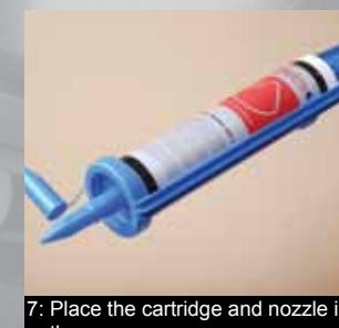
7: Place the cartridge and nozzle in the grease gun
