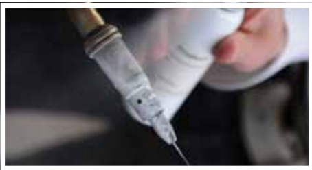
Apply Weld-max A on welding torch
